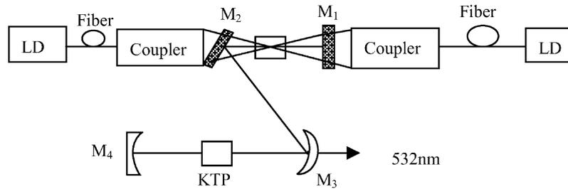
Fig. 1. Experimental setup of LD two-end-pumped Nd:YVO<sub>4</sub> laser.
