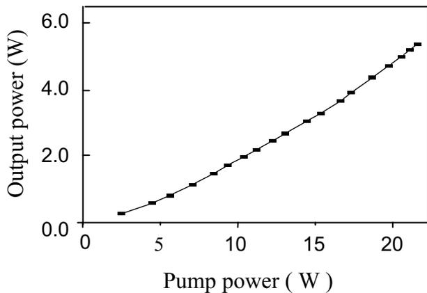
Fig. 3. 532-nm laser output power as a function of diode-laser pump power.
