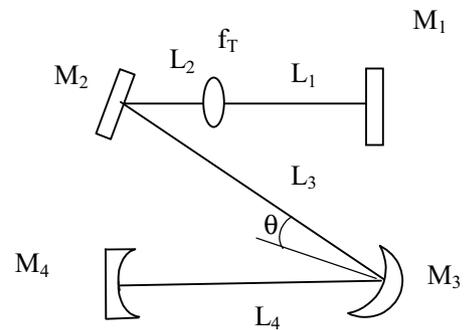
Fig. 2. The corresponding thermal lens equivalent resonator.
